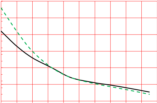
FIG.7: Relative variations of gate trigger current, holding current and latching current versus junction temperature
