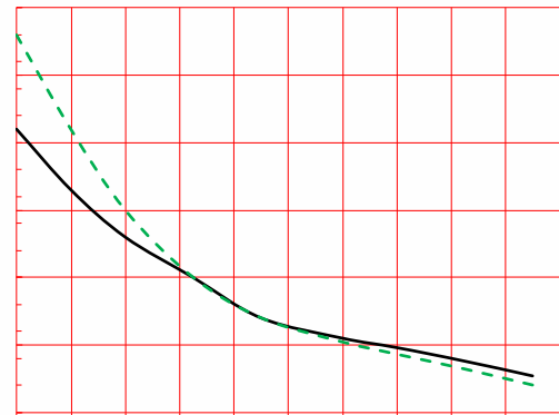
FIG.6: Relative variations of gate trigger current, holding current and latching current versus junction temperature
